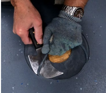
Using an angled skiving knife
